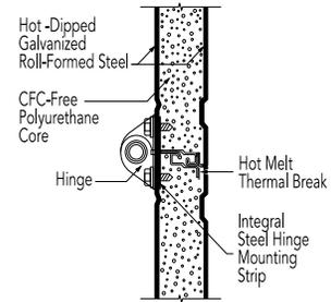
The Thermacore® steel-polyurethane-steel sandwich panel construction is lightweight, incredibly strong and exceptionally efficient – reflecting a premium level of thermal performance.
